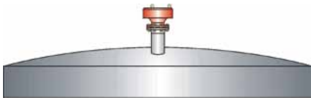
Figure 1: Free venting of the storage tank with PROTEGO® EH/OS
