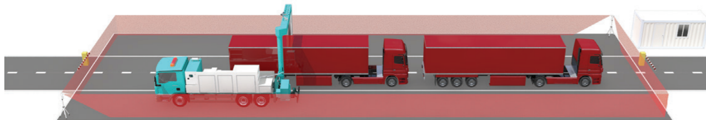
2. Sequential scanning of a number of vehicles placed in a line for a higher throughput;
