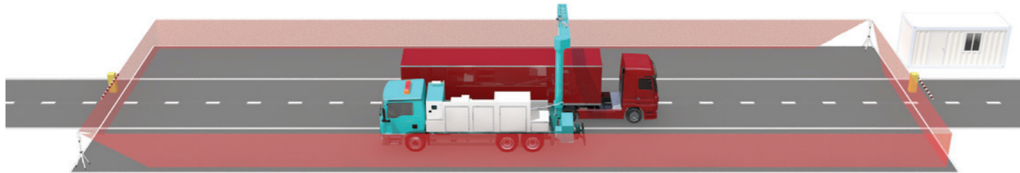
1. One by one scanning of stationary vehicles (optimized solution in terms of penetration and image);
