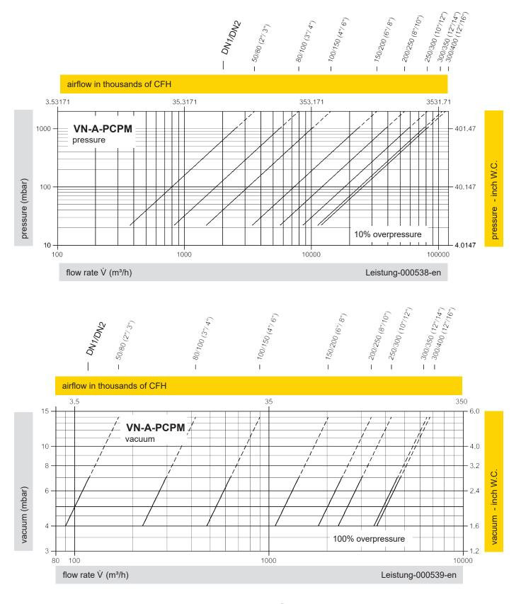
The flow capacity charts have been determined with a calibrated and TÜV certified flow capacity test rig. Volume flow  $\dot{V}$  in (m<sup>3</sup>/h) and CFH refer to the standard reference conditions of air ISO 6358 (20°C, 1bar). For conversion to other densities and temperatures, refer to Sec. 1: "Technical Fundamentals".
